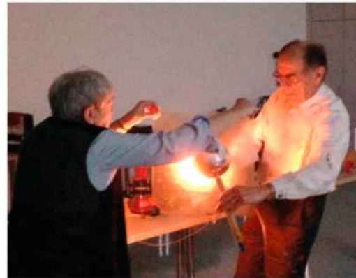
Fig. 21. Demonstration of a propagating brush discharge at a bipolar charge layer by Günter and Sylvia Lüttgens [11, page 167]. In this case, this highly insulating film carries the bipolar charge only in the center region, so it can be held by hand, as shown in the picture.
